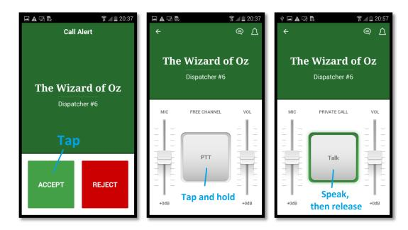
Figure 23: Responding to a call alert: accept (left), call (middle), speak (right)
